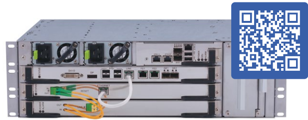
Dunay unit designed in 3U chassis for a telecommunication rack
